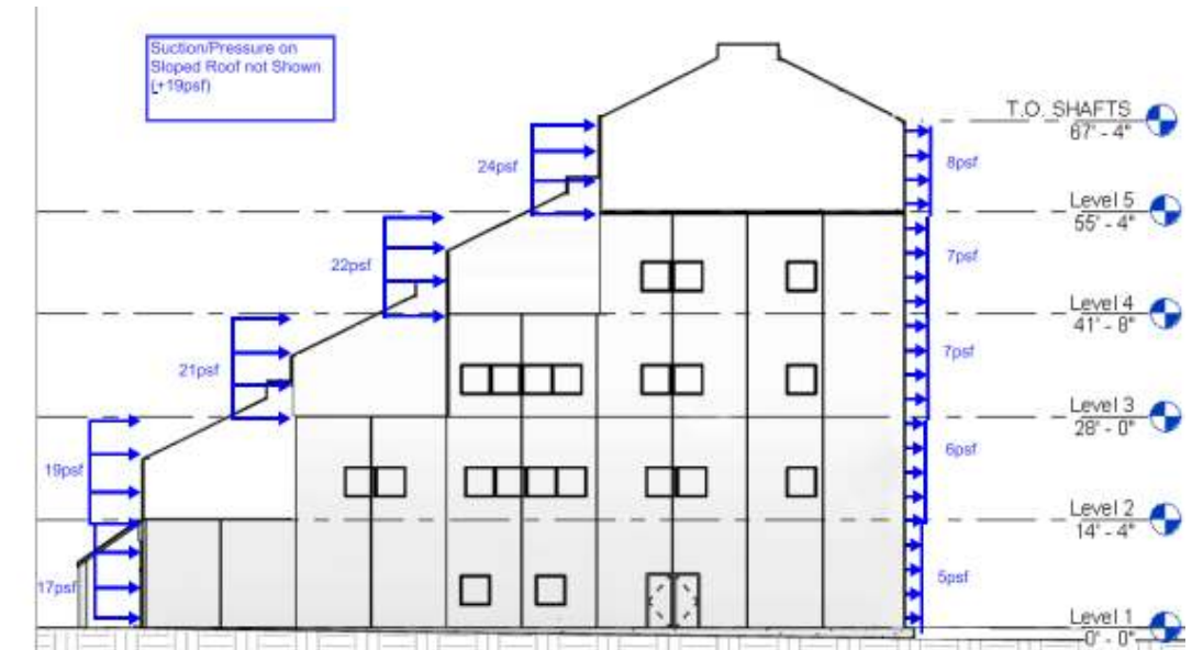
FIGURE S.2: WIND LOADING PRESSURES FOR MILWAUKEE
